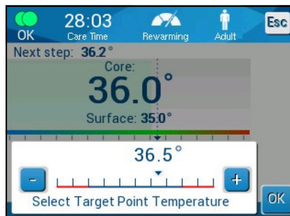
Figure 28: Target Temperature Setting Panel
