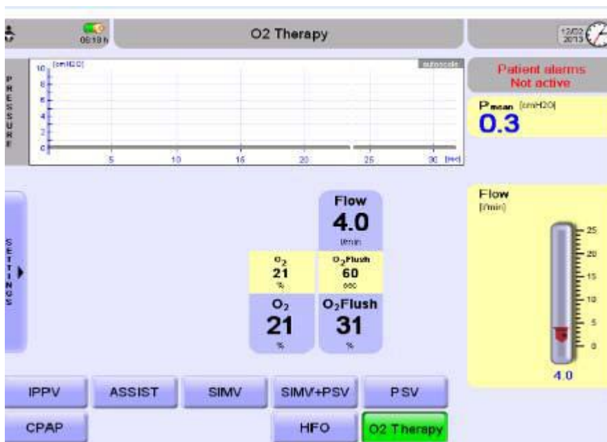
Fig 3 – High Flow Screen on Fabian ventilator
